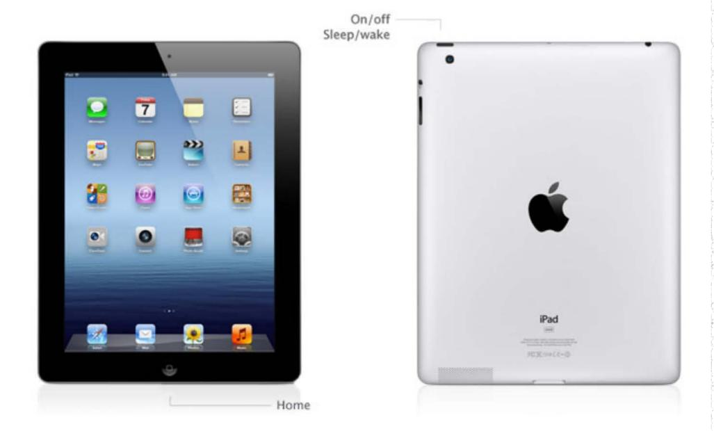
In the image above, look at the two buttons: the one on the front, below the screen, is the Home button. The one on the top, on the backside of the bezel, is the Sleep/Wake button. Press both buttons at the same time and you will hear the Camera sound and see the screen go white for just a second. That's all there is to it – your screen is now captured.
